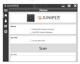
Note: You can also test the scan function by putting the cursor in **Scan Data** and pressing the keypad button assigned to RFID scanning.
